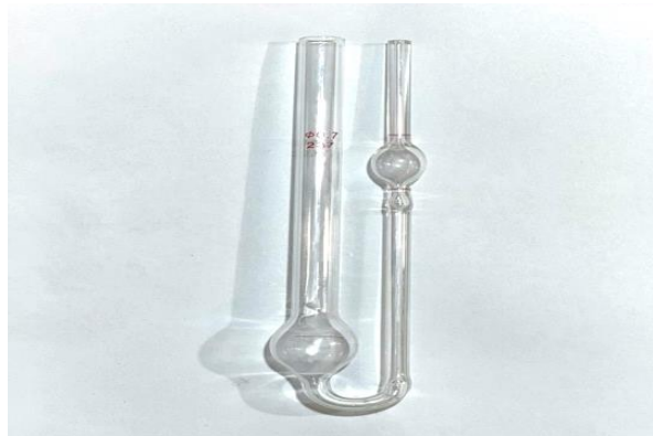
Fig (5): Ostwald viscometer used for viscosity measurements.
